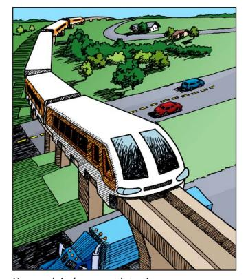
Some high-speed trains run on electromagnets. The trains have powerful electromagnets on the bottom. The track also has powerful electromagnets. The two electromagnets face each other so that they repel each other. The magnetic force is so strong that it lifts the train off the track. The train floats above the track. It actually flies as it travels. This makes a fast, smooth ride.
